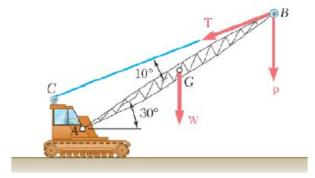
Plot the tension and reaction at A as a function of boom angle from 0 to 90 degrees taking the weight of the boom to be 5.2 kips and the lifting load to be 20.6 kips. Before plotting these data, you may check your program by solving the problem given by McGraw-Hill Connect.
